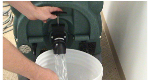
Draining the Recovery Tank
